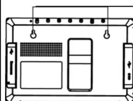
Mount the device onto the screws securely applied on wall.
