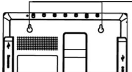
Mount the device onto the screws securely applied on wall.
