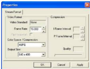
Click on **Video Capture Pin** to adjust video streaming parameters. Adjust **Output Size** to best resolution desired.
