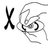
Do not wipe in a circular motion (concentric scratches on the disc surface tend to cause noise). Gently wipe from the center of the disc to the outer edge as the right figure.
