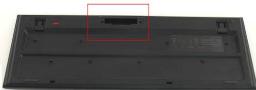
2. Install the batteries into keyboard and mouse as illustrated. Please match up polarity signs on batteries and devices.
