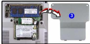
4. Gently pull the two release latches (4) & (5) on the sides of the memory socket.
