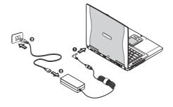
2. Connect one end of the AC adapter to the DC-in port on the computer's rear panel (1);connect the power cord to the AC adapter (2) and the other end to a properly grounded power outlet (3).
