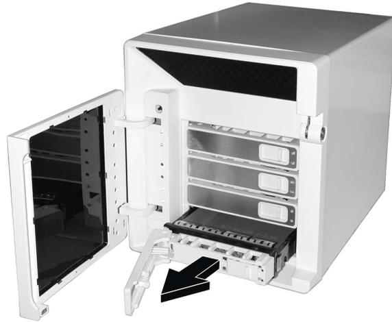
4. Unfasten two screws from each side of the hard disk tray and remove the metal bracket.
