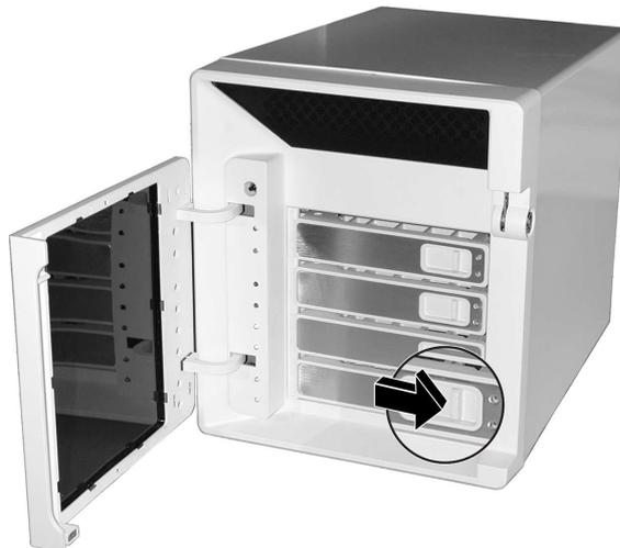
**NOTE:** Install the first hard disk on the lowest level tray, the second hard disk on the second lowest level tray, and so forth.
