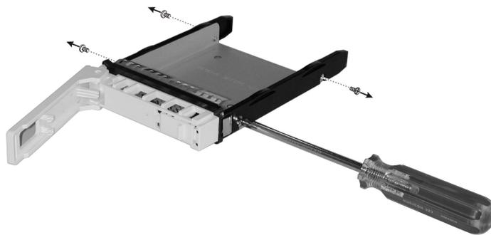
5. Fit the hard disk into the tray with the connectors pointing toward the rear. Then align and fasten four screws to secure the hard disk in place.
